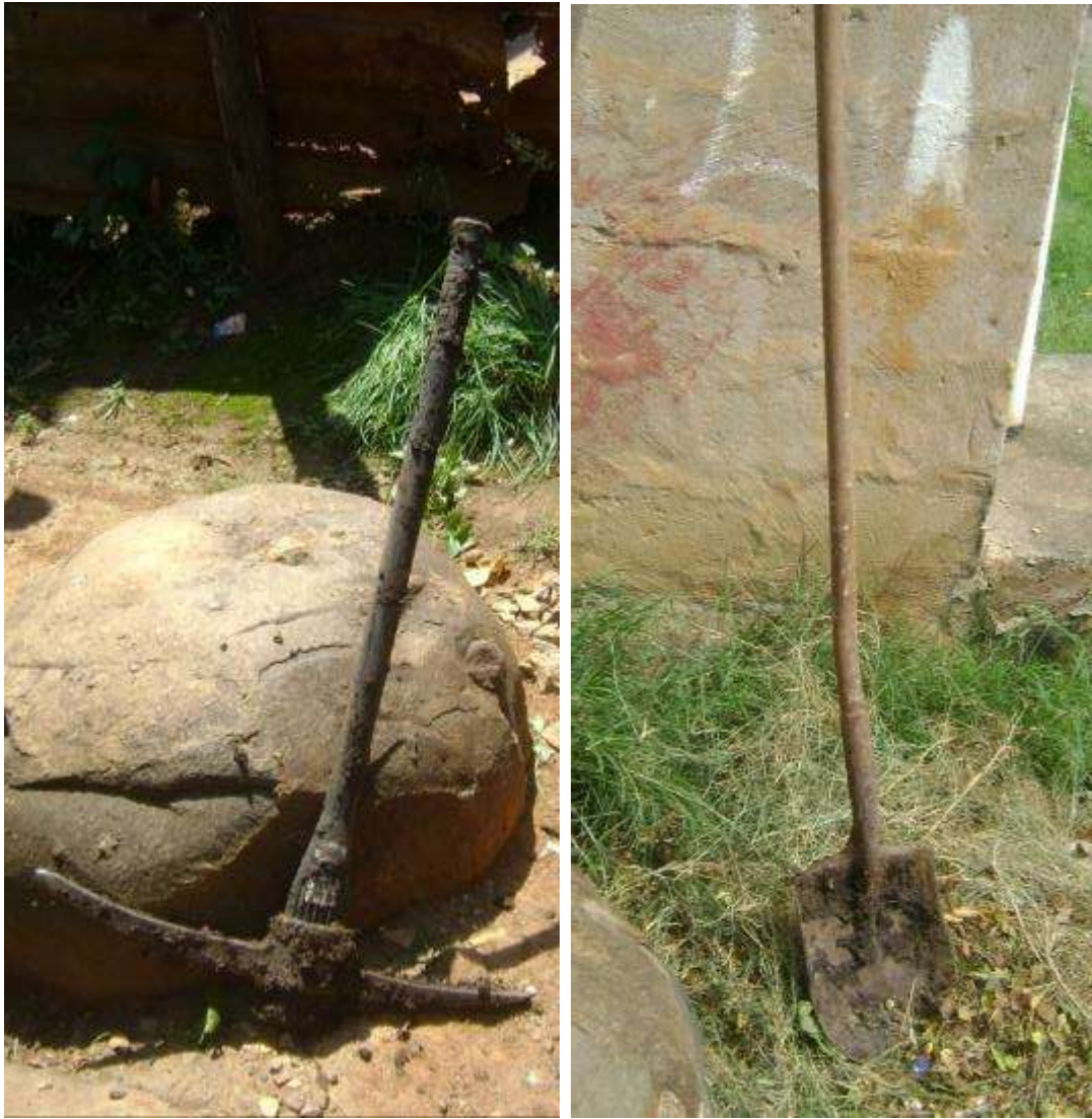
Figure 18 Workers had no option but to place contaminated tools on household surfaces, thereby contaminating them, as they carried no tarpaulins with them on which to lay their tools.
