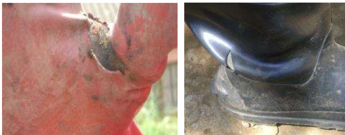
Figure 8 A torn glove (left) and boot (right) which no longer provide an effective barrier between skin and sludge.
