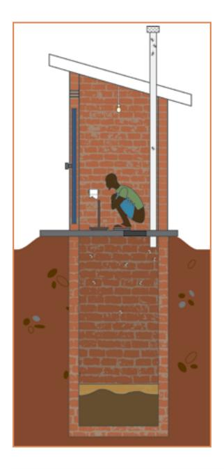
Lined pits and septic tanks can be emptied safely and will prevent faecal sludge from entering the environment and contaminating ground water or water sources around you, protecting your health.
