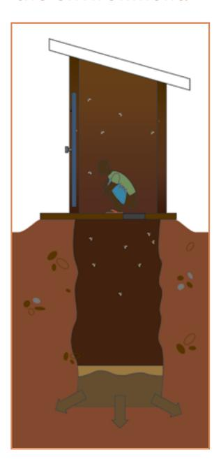
The faecal sludge can enter through the soil and stones and easily contaminate the ground water and water sources around you thus posing a threat to your health.
