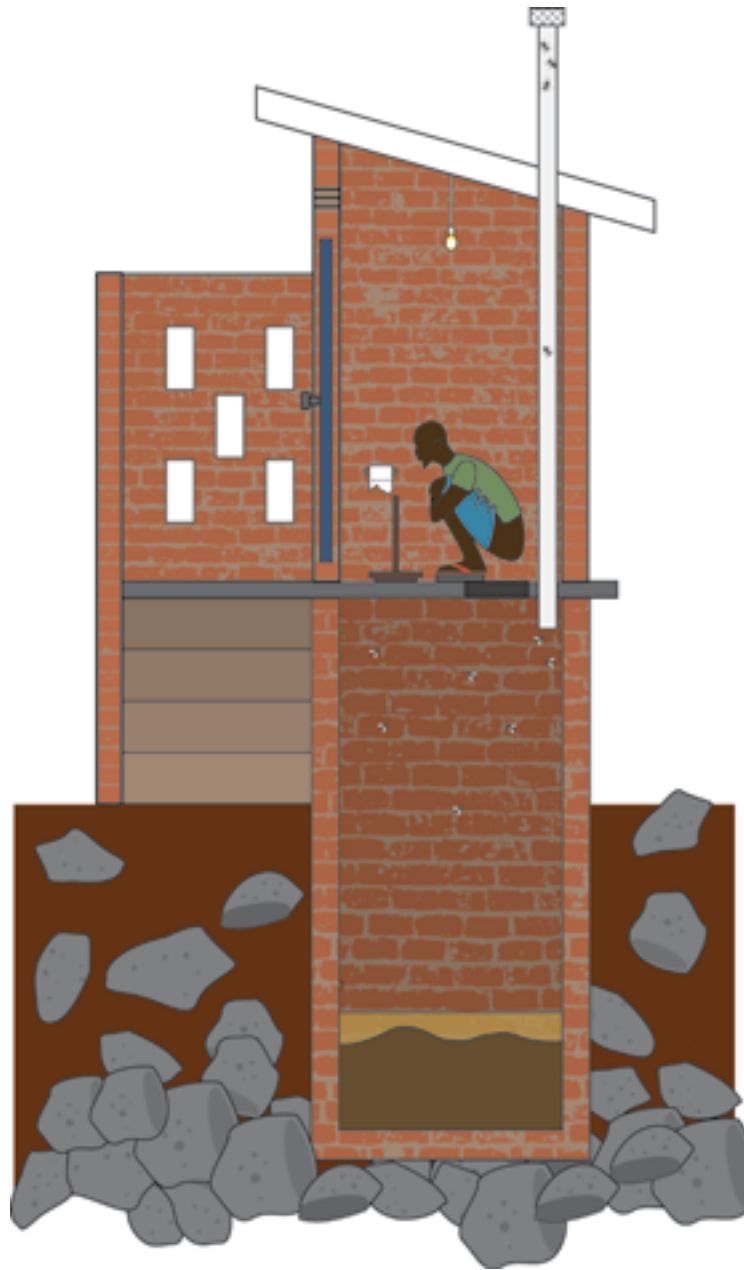
FIGURE 2-5 RAISED VENTILATED IMPROVED PIT LATRINE & INTERIOR DETAILS
