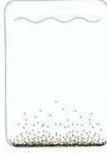
secondary settling tank
