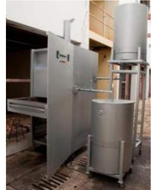
Waste oil regeneration kiln, Dakar Pellets and briquettes
