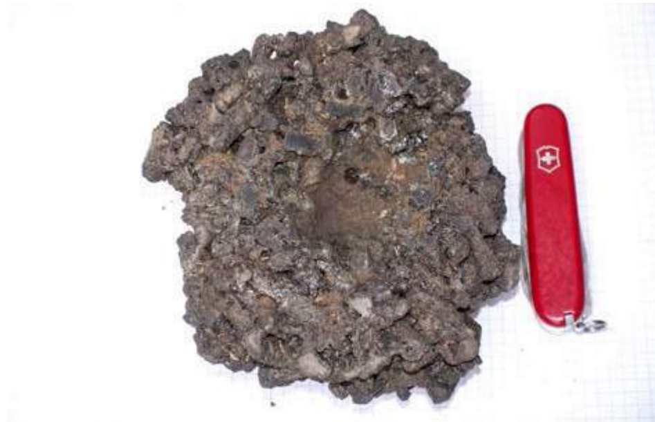
Clinker deposit from gasifier
