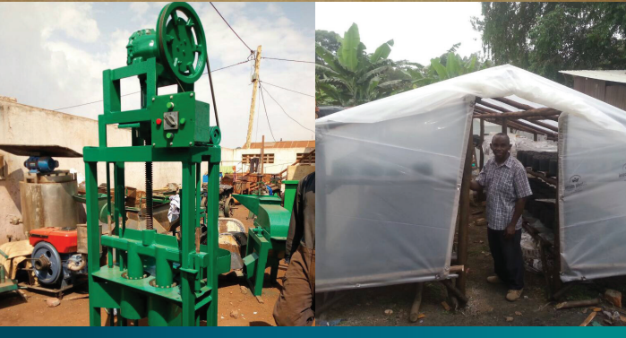
Clockwise from top: RRR entrepreneurs complete a training module; plastic sheet greenhouse speeds up the briquette drying process; mechanized briquette-making machine
