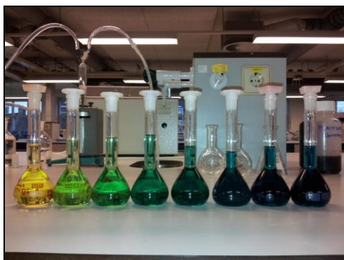
Figure 5-3 Preparation of ammonia-nitrogen calibration curve
