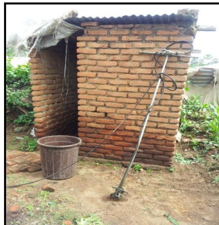
Figure 7-2 Spray nozzle used for faecal sludge fluidisation
