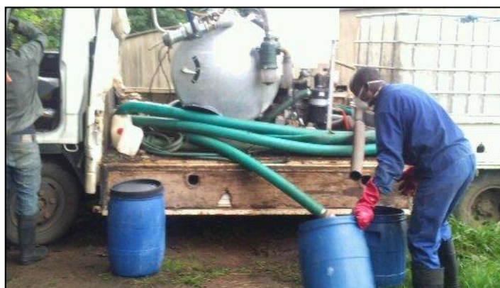
Figure 5-5 Filling of drums with collected faecal sludge
