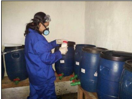
Figure 5-6 Addition of urea to faecal sludge
