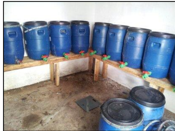
Figure 5-7 Reactors used for the urea treatment
