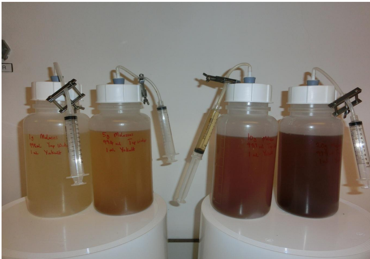
Figure 4.1 Miniature batch reactors for Lactic acid bacteria (LAB) proliferation in molasses-tap water
