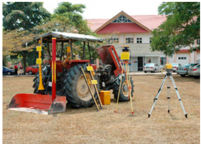
Fig. 6: Laser-guided land levelling technology has improved surface irrigation, particularly in rice basin areas
