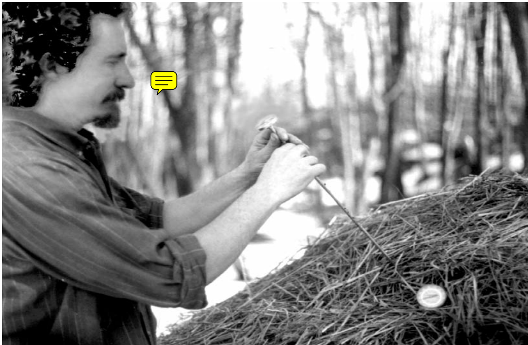
Figure 3.2: The author probing a humanure compost pile in late winter. This compost had not yet become thermophilically active. Of the two thermometers, one has a long probe and the other a short one.
