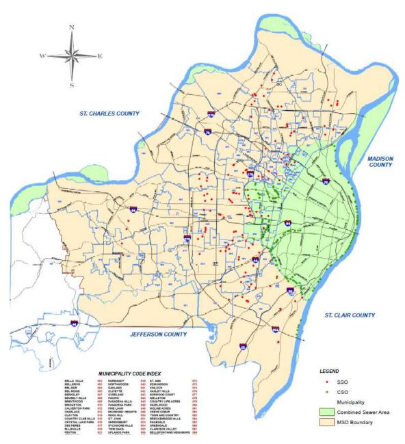
Figure 2: MSD Constructed Sewer Overflows Map (http://www.stlmsd.com/sites/default/files/education/ConstructedSewerOverflows 04112016.pdf)
