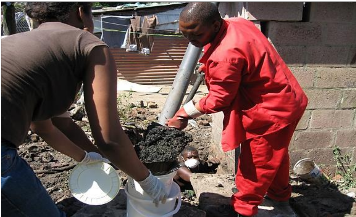
Figure 3-1: Photograph showing the collection of samples during a pit emptying exercise
