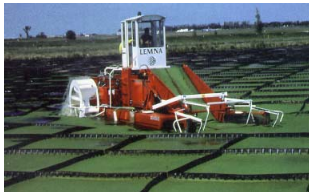
Photograph 13: Diesel-powered mechanical harvester for biomass removal in larger duckweed-based wastewater treatment lagoons in the USA. (Photograph: Lemna Corp. 1994).
