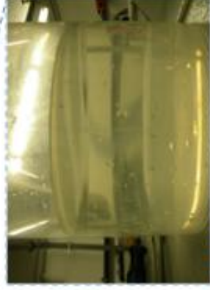
6 - Permeate Treated brownwater, COD: ~ 18 mg/l
