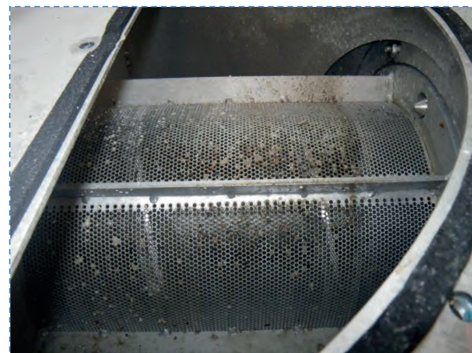
2 - Screen basket with screw For solids separation (hole size: 3 mm)
