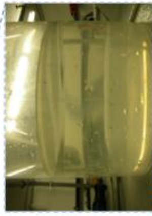
6 - Permeate Treated brownwater, COD: ~ 18 mg/l
