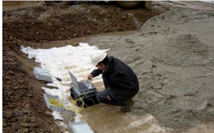
Controlled measuring on an area of sensor-based geotextile as part of the application process: field test in Swienna Poremba (Poland)
