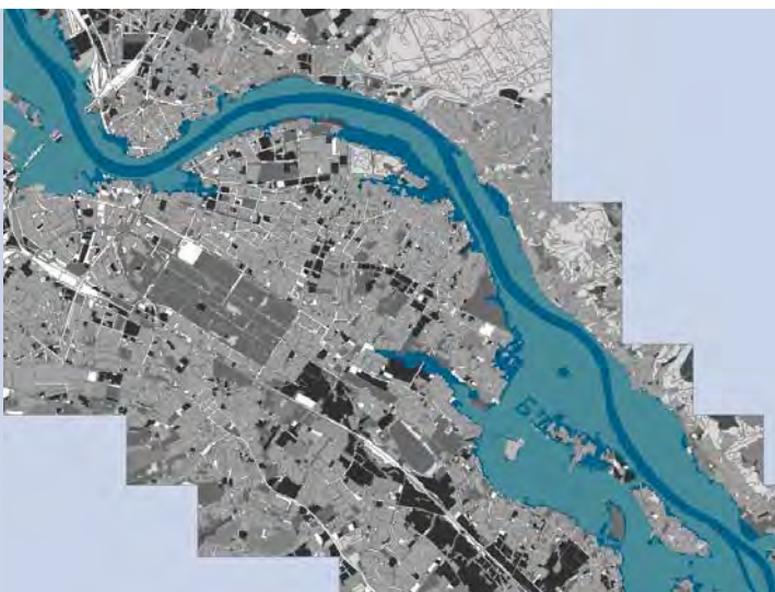
Advance calculation of flooded surface areas through realistic modelling (Map background source: city of Dresden)
