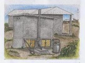
It is low cost in construction and does not require excavation of pit during construction
