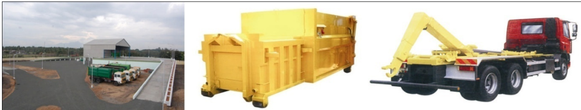
Figure 54 Equipment at Transfer Station - Stationary Compactor and Large Hook Loader Vehicle for Transfer Stations
