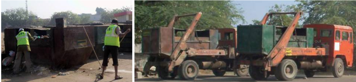
Figure 37 Fleet for Transportation of MSW from Secondary Collection Bins
