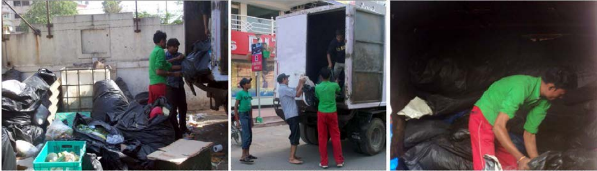
Figure 50 Inappropriate fleet design - Inconvenient loading (left & centre); Manual stacking of garbage bags (right)
