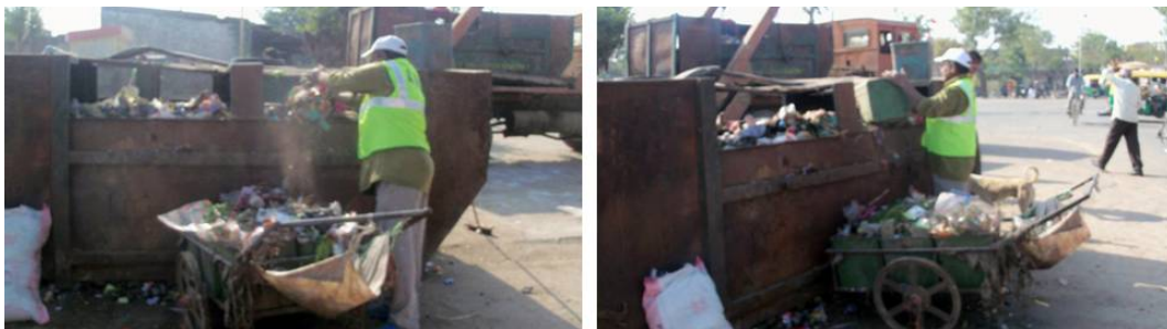
Figure 48 Manual Emptying of Street Sweeping cart (left); High opening of Secondary Bin (right)
