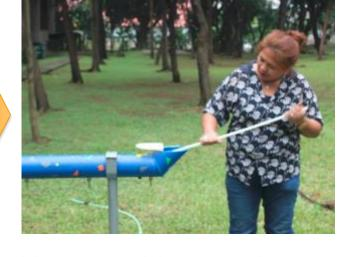
Requires tilting the water container to access the opening and a wrench to open the plug on the pipe
