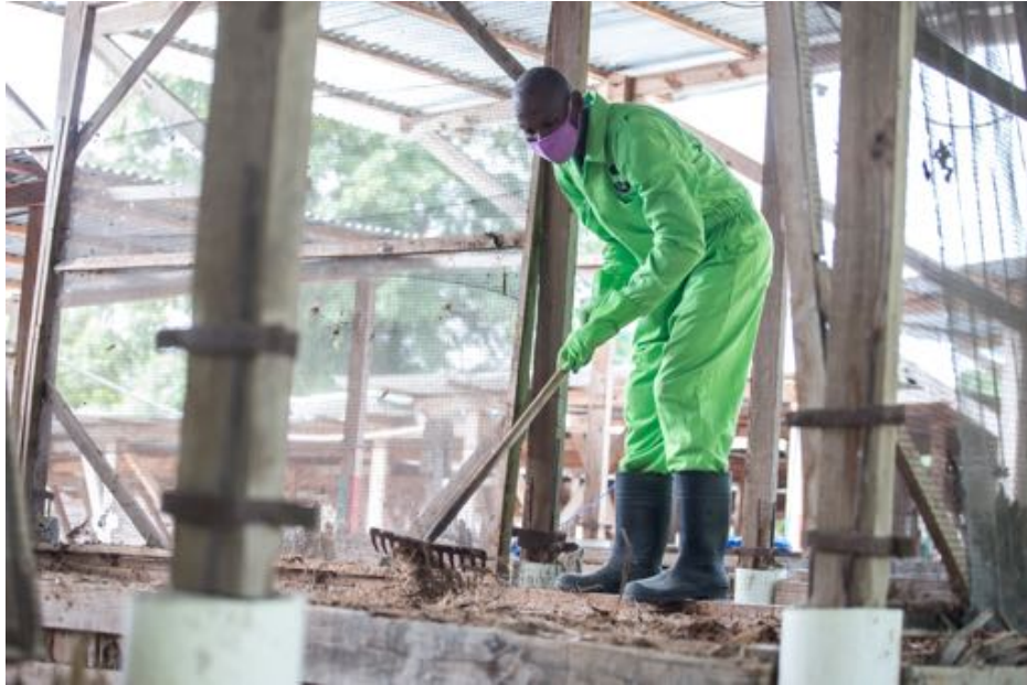
Wearing protective gear, a worker at the composting facility rakes cover material over a newly filled compost bin. Photo: Caleb Alcénat/Labelimage for Project #WasteNot (CC BY-NC-ND 4.0).
