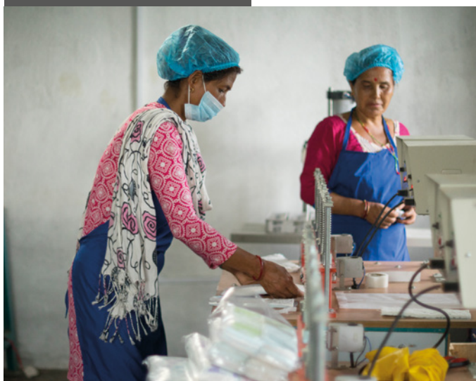
Employee operating the shortening and sealing process machine // Figure 15
