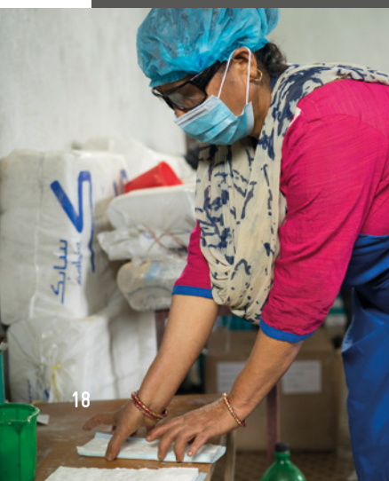
Gluing the polyethylene film and the basis of the pad together // Figure 14
