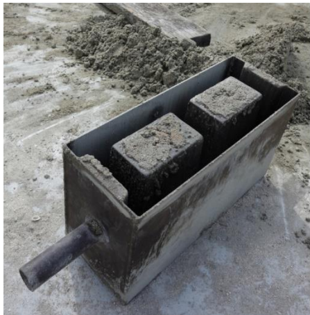
Figure 25: Mould and self-made cellular concrete blocks.
