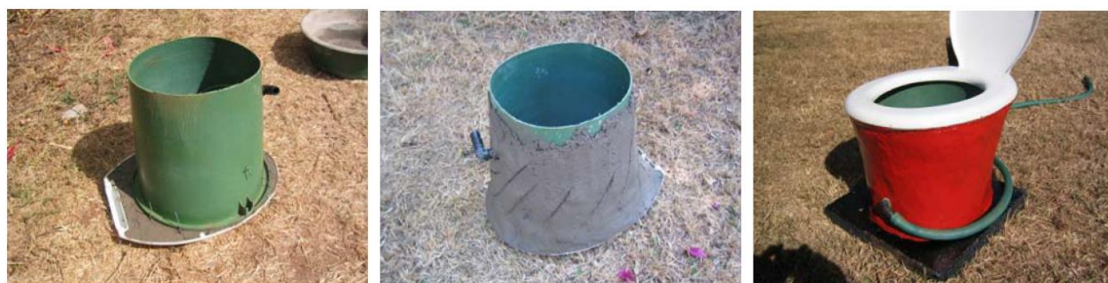
Figure 18: Construction of low-cost UDDT pedestal (Morgan, 2007, p.51, 53, adapted).
