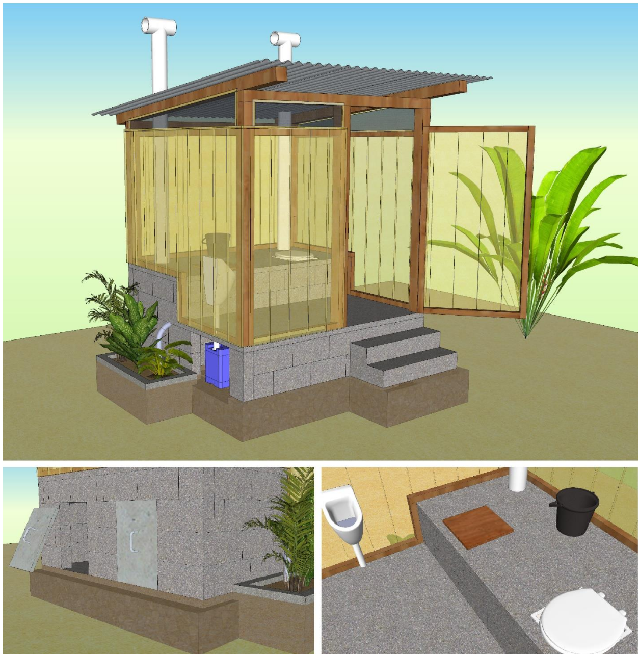
Figure 24: Drawing of Urine-Diverting-Dry Toilet.
