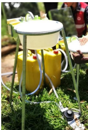
Figure 27: Jengu connected to jerry cans filled with water; variations of the Jengu handwashing device (left to right: for people with reduced mobility, children and adults) Credit: G. Rose, British Red Cross; Arup
