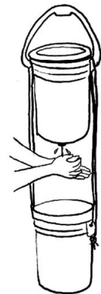
Figure 14: The Tap Up – a two bucket hand sink . Credit: Lippincott (2011), CERN Open Hardware Licence
