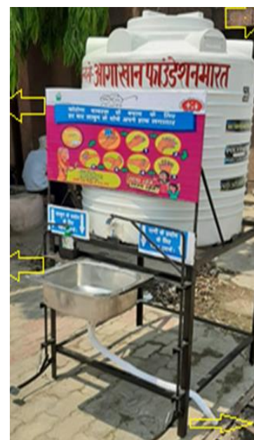
Figure 17: pedal operated handwashing station with large tank. Credit: Aga Khan Foundation, India
