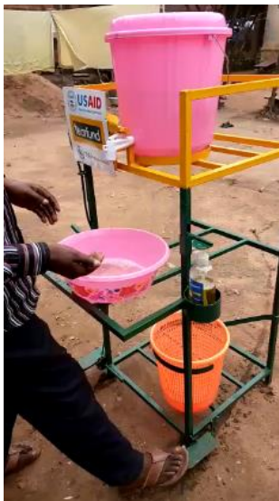
Figure 19: pedal-operated handwashing station. Credit: Tearfund DRC
