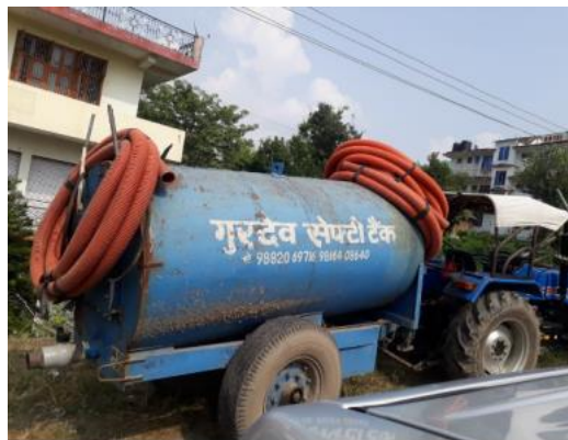
Figure 4: Truck-mounted vacuum tanker (Source: Saiyami/CSE, 2020).
