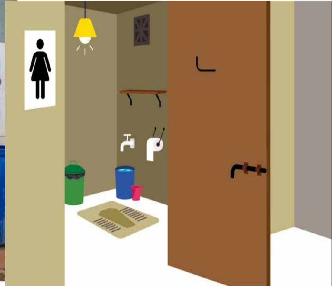
Figure 3: An example of the interior of a female-friendly toilet cubicle.
