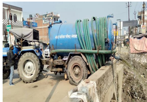
Deslugger emptying septage into nullah
