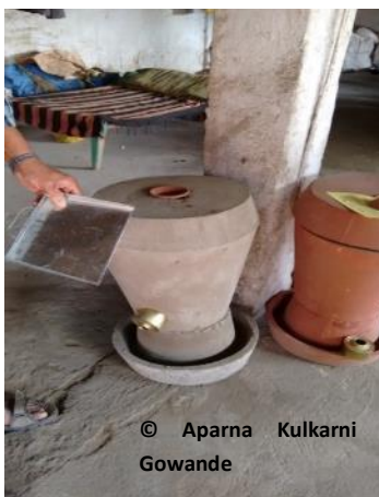
Figure 3: Low-cost incinerator in an earthen pot
