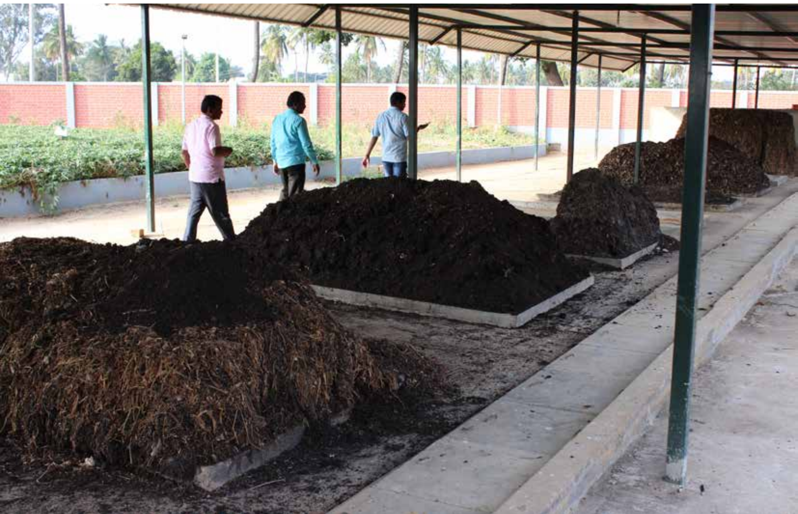
Figure 4 - Co-composting unit set up in the extra land that was allocated during the design phase
