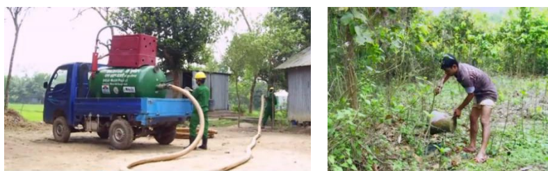
Figure 3: Vacu-tug (transports FS to treatment plant) and dumping FS in open ground.
