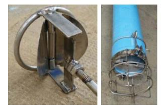
of PVC riser pipe containing two stainless non-return butterfly valves. The Gulper is a recent invention which is inexpensive and easy to operate. Adverse health impact is significantly reduced as there are very less chances of sludge contact. The Gulper can be built using locally available material and manufacture techniques, even those which are common in low-income countries. This technology is very much suitable for densely populated and low-income areas.
