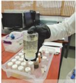
3. Shake sample until reagent is completely dissolved.
