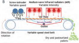
**Figure 4.21** A) the laboratory-scale LaDePa, and B) a corresponding schematic representation of the process (photo and schematic: UKZN PRG).
