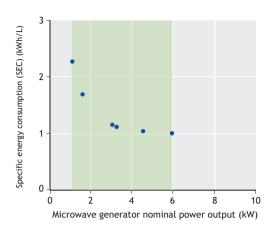
Figure 4.26 Effect of microwave generator power output on the specific energy consumption (SEC) (Kocbek et al., 2020).
