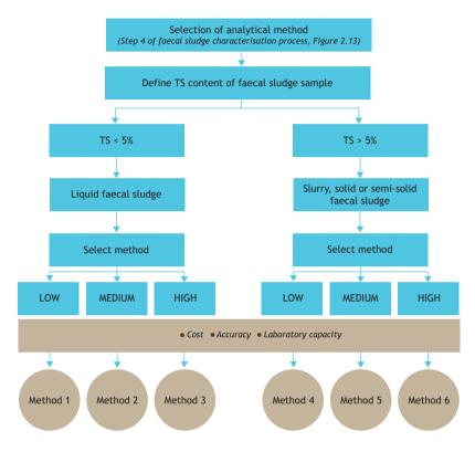
**Figure 2.14** An example of a decision-making tree for the selection of a method of analysis depending on the purpose of characterisation. Step 4 refers to Figure 2.13, Steps in the faecal sludge characterisation process. Note: This example is specific to methods that differ for less than or are greater than 5% TS.
