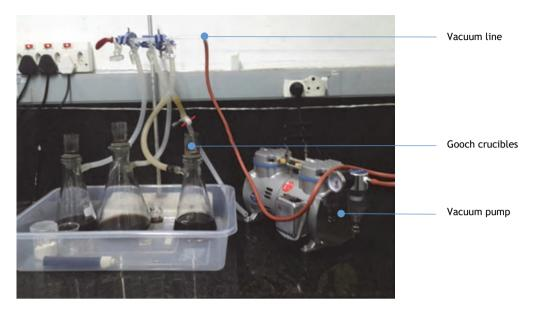
Figure 8.6 Vacuum filtration setup (photo: UKZN PRG).
