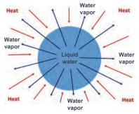
**Figure 4.14** Schematic representation of drying faecal sludge. Red arrows represent heat transfer, blue arrows represent mass transfer of water (H<sub>2</sub>O).
