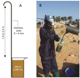
**Figure 3.8a** A) schematic of the grab sampling beaker device. B) at the outlet of the Cambérène FSTP, ONAS staff, Dakar, Senegal. Note: wide-mouth containers are preferable for sample allocation, as they aid sample collection without spillage (photo: Eawag).
