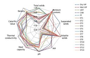
**Figure 7.8** Comparison between different properties of faecal sludge with the synthetic simulants to establish which of the developed simulants had the best match with faecal sludge from different onsite sanitation facilities.
