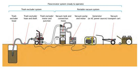
Figure 2.8 Innovative technology for faecal sludge emptying - the Flexcrevator (source: North Caroline State University<sup>4</sup>).
