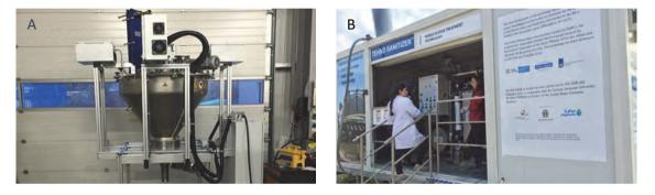
**Figure 4.18** A) the bench-scale Shit Killer microwave-based technology for sludge treatment developed by IHE Delft and Fricke und Mallah Microwave Technology GmbH, and B) the follow-up prototype – the pilot-scale Tehno Sanitizer developed by IHE Delft and Tehnobiro d.o.o. (photos: IHE Delft).
