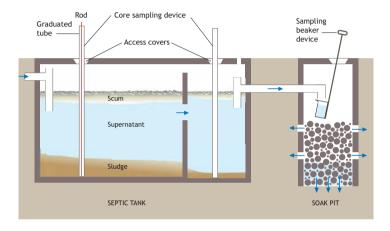
**Figure 3.14** Sampling points in a septic tank: on the left is a vertical core sample in the first chamber, in the middle is a vertical core sample in the second chamber and on the right is a grab sample of the septic tank effluent (depending on configuration, e.g a distribution box or open drain).
