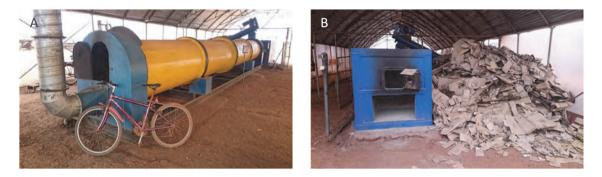
**Figure 4.15** A) a rotary convection dryer operated by Pivot, in Kigali, Rwanda and B) waste cardboard is burned in a boiler and the hot gases produced are used as the heat source for drying. The sludge is pre-dried by a solar dryer before entering the convective dryer pictured here (photos: UKZN PRG).
