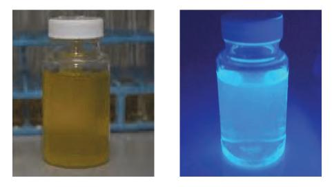
Figure 8.24 Control sample for Total Coliforms (left) and fluorescent control sample of E. coli (right) (source: UKZN PRG).
