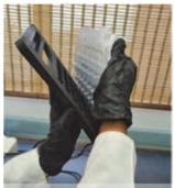
7. Hold rubber frame upright with one hand and place the tray against the frame to fit into the slots.
