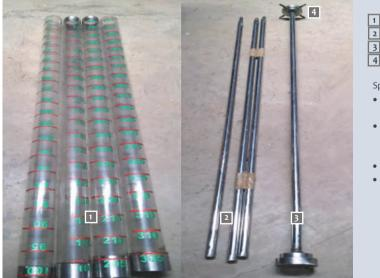
Core sampling tubes that fit together Rods that screw together inside the tubes Air-tight seal to close bottom tube Locking system to attach to top-most rod
