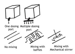
**Figure 4.11** Diagram representation of the different conditioner dosing and mixing configurations evaluated by Sanivation.
