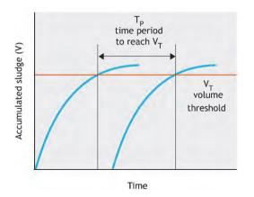
**Figure 3.12** The blue lines illustrate change in the faecal sludge accumulation rate and  $T_P$  is the amount of time to reach  $V_T$ , the volume threshold where emptying is triggered.
