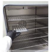
9. Incubate trays at 35 °C for  $18 \pm 4$  h for Total Coliforms and *E. Coli* pr at 44 °C for  $18 \pm 4$  h Faecal Coliforms.
