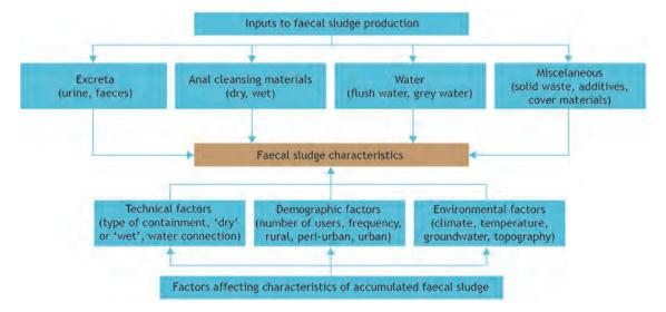
**Figure 2.2** Illustration of the inputs to faecal sludge described in Section 2.3.1, and different technical, demographic, and environmental factors affecting and modifying the characteristics of faecal sludge in onsite containment, as described in Section 2.3.2.
