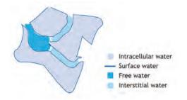
Figure 4.1 Representation of the different forms of water in a sludge floc (adapted from Bassan *et al.*, 2014)
