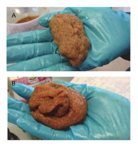
Figure 7.3 Simulants with 30 wt % of solids content yeast extract and no baker's yeast: A) SE65; B) SE80.
