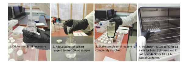
Figure 8.23 Procedure for Presence/Absence (P/A) test for total coliforms and E. coli and Faecal Coliforms (source: UKZN PRG).
