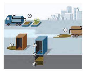
**Figure 5.5** Illustration of six stages for mass balance calculations: 1. excreta production; 2 faecal sludge production; 3. faecal sludge accumulation; 4. faecal sludge emptied, not collected; 5. faecal sludge collected, not delivered to treatment; and 6. faecal sludge collected, delivered to legal discharge/treatment (image: Strande *et al.*, 2018).
