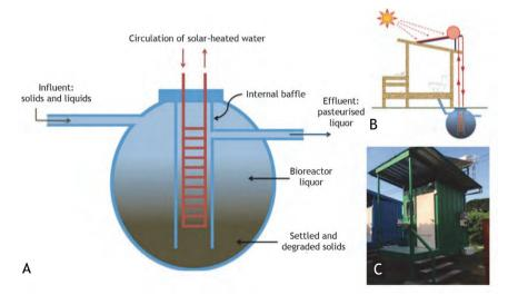
**Figure 2.6** Principles of the Solar Septic Tank: (A) principles of solar heating applied to SST; (B) illustration of the buried septic tank and solar collection unit on the toilet roof; (C) installation of the SST in the field test site (source: AIT).
