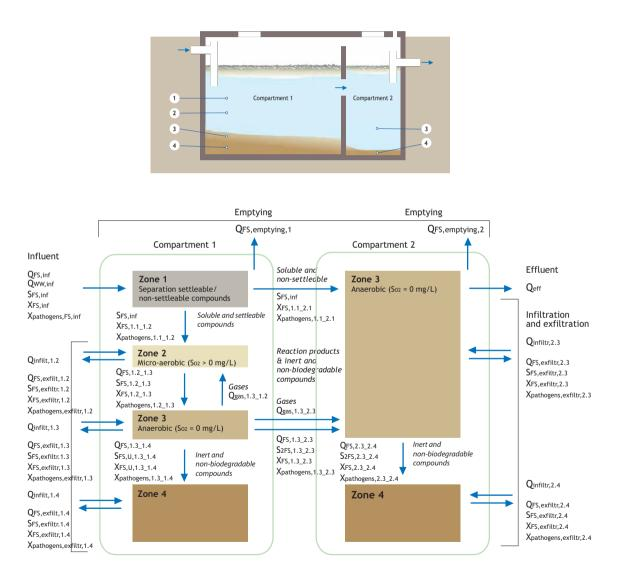
Figure 6.9 Septic tank: suggested model structure.
