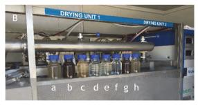
**Figure 4.24** A) an experimental microwave-based faecal sludge drying unit, and B) samples taken at different points in the process: a) filtrate from the sludge press, b) concentrated sludge from the sludge press, c) ultrafiltration concentrate, d) ultrafiltration permeate, e) reverse osmosis concentrate, f) reverse osmosis permeate, g) dry sludge, and h) condensate (photo: IHE Delft).
