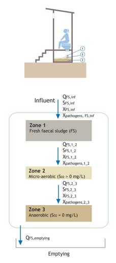
Figure 6.7 Portable toilet: suggested model structure.
