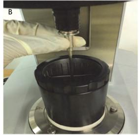
**Figure 8.15** Loading the sample into the cone cup and then to the plate (A), and attaching the measuring system to the adapter (B) (source: UKZN PRG).
