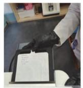
8. Feed the trey into the sealer and collect sealed tray at the bottom end.
