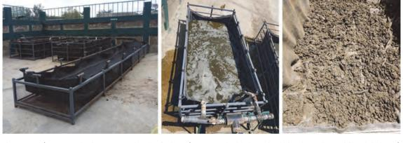
Figure 4.10 A) a geotextile skip setup at the pilot facility; B) a geotextile skip being loaded with conditioned faecal sludge; C) dewatered sludge ready to be unloaded from a geotextile skip (photos: Sanivation).
