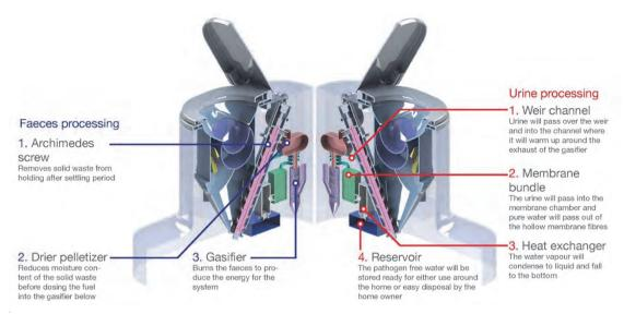
Figure 2.5 Nano Membrane toilet: an example of a waterless self-contained toilet (source: Cranfield University<sup>3</sup>).
