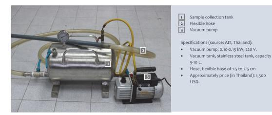
Figure 3.5 Vacuum sludge sampling device (photo: AIT).
