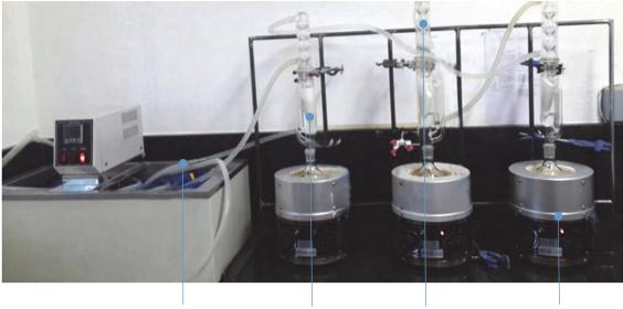
Cooling water for circulation in condenser Soxhlet with thimble Condenser
