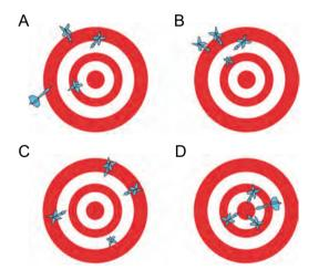
**Figure 8.1.** Dartboards showing different accuracy and precision scenarios. A: neither accuracy, nor precision; B: precision (close repetitions) but not accuracy; C: accuracy but not precision; and D: both accuracy and precision (required result of QC measures). Source: Byron Inouye, 2020.
