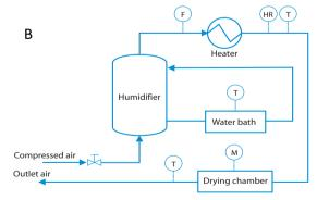
**Figure 4.19** A) the custom-designed convective drying rig (photo: UKZN PRG) and B) a schematic representation of the convective drying rig, F: air-flow measurement; T: temperature measurement; M: mass measurement; HR: relative humidity measurement.
