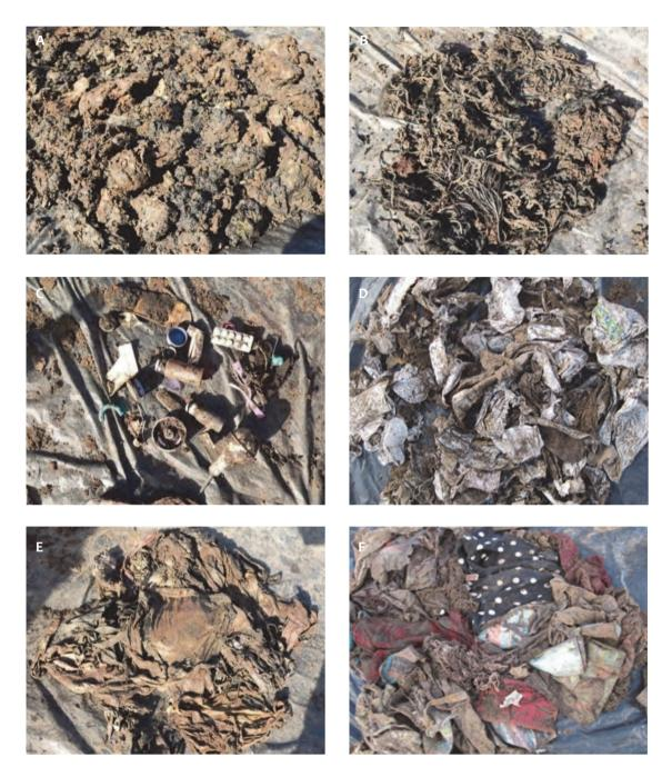
**Figure 2.3** Solid waste materials removed from onsite containments in Durban, South Africa: A) paper, B) artificial hair, C) rigid plastics, D) menstrual products and nappies, E and F) textiles (A, B, C and E are from ventilated improved pit latrines; D and F are from a standing UDDT vault, not currently in use), (source: UKZN PRG).
