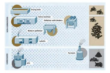
**Figure 4.13** An overview of technology options for producing solid fuel, starting from dewatered faecal sludge at 80% moisture and ending at non-carbonised or carbonised solid-fuel end products. The position of the technology icons from left to right indicates the required dryness of the input sludge for each technology, as indicated by the size of the droplets, ranging from 80% moisture on the left to 10% moisture on the right (modified from Andriessen *et al.*, 2019).
