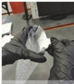
5. Poor the sample into the Quantitray
