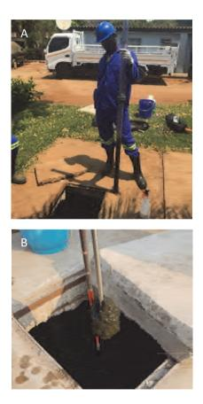
**Figure 3.3** A) taking a core sample from a septic tank in Lusaka, Zambia, and B) the sampling device becomes clogged if the sludge is too thick. This example shows the collection from a 10-year old septic tank that had never been emptied. The tank was leaking, and so the supernatant leached out into the soil, resulting in a very thick sludge accumulation (photos: Eawag).
