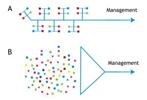
**Figure 5.1** A) schematic of wastewater transported through sewer to treatment plant, where it is somewhat homogenised during transport. Squares represent level of each individual connection (*e.g.* household, business). B) schematic of faecal sludge, which is collected, transported, and delivered to treatment plant at the level of individual, onsite containment, without homogenisation. Shapes also represent level of individual onsite containments.
