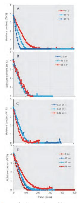
**Figure 4.20** A) Drying rate as a function of air temperature, B) relative humidity, C) air velocity, and D) pellet diameter.
