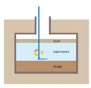
**Figure 3.2** L-stick measuring device for depth of layers in a septic tank.
