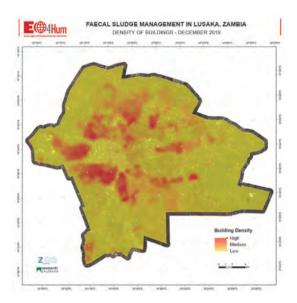
**Figure 5.14** Building density in Lusaka, Zambia (map generated by Johannes Nödel and Barbara Riedler). Density calculations were based on data integration of building footprints derived through (*i*) semi-automated, object-based extraction using a very high resolution Pleiades satellite imagery from 2018, (*ii*) OpenStreetMap, and (*iii*) field data provided by GIZ. Values of building density range from low (o buildings/ km<sup>2</sup>) to high (4,800 buildings/km<sup>2</sup>).
