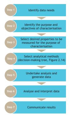
**Figure 2.13** Steps in the faecal sludge characterisation process. Further information on how to select analytical methods (Step 4) is provided in Section 2.4.2. Further information on the integrated approach for data collection, analysis and interpretation within the entire book is provided in Chapter 1, and further information on integrating characterisation into a sampling plan is included in Chapter 3.
