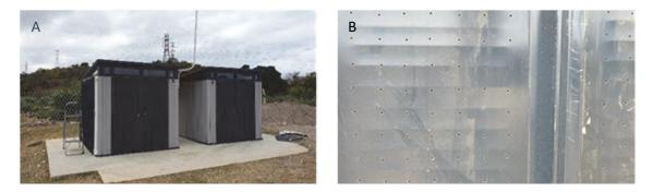
**Figure 4.17** A pilot-scale solar dryer developed by Swansea University and tested in Durban, South Africa. A) sludge is placed inside these sheds to dry. B) the walls of the sheds absorb solar energy and transfer it to the sludge inside through a ventilation system (photos: UKZN PRG).
