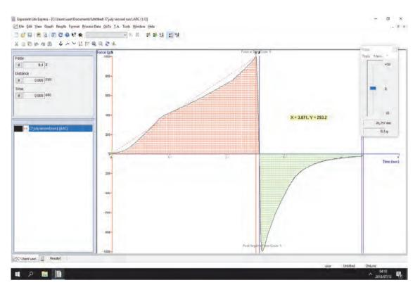
Figure 8.18 Typical graph of a test with the red part showing the compression forces and the green part showing the tension forces.
