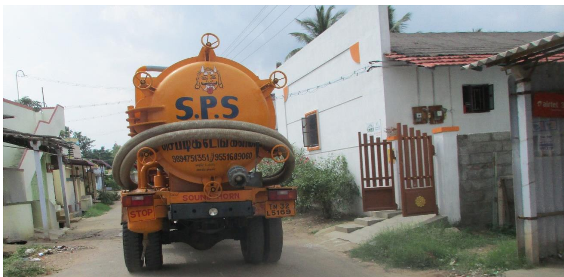
Figure 4.12: Desludging truck in Town Panchayat
