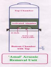
filter controls the flow rate and ensures sufficient bed contact time. The filtered water gets collected in the bottom container. AA gets exhausted after a certain time and will need to be regenerated periodically. The periodicity will depend on the chemical composition of raw water and allowable maximum permissible limit of arsenic in
