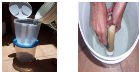
Fig 4: Filling the filter and cleaning the ceramic candle
