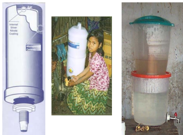
Fig 3: Ceramic candle filter designs - Photos courtesy of Tom Clasen LSHTM
