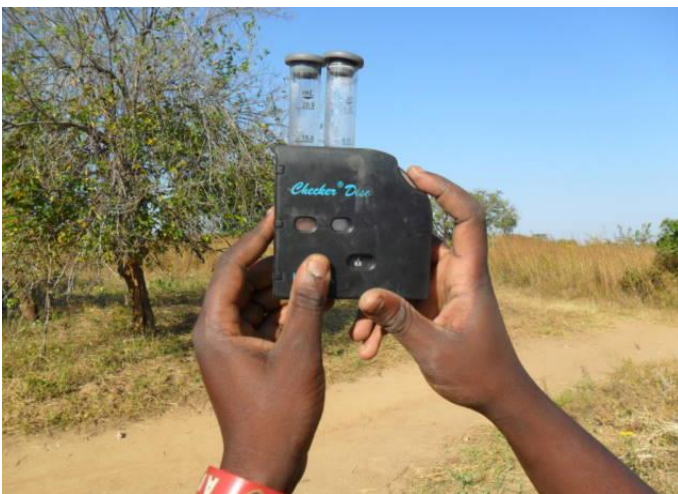
Figure 10: Checking iron content at the wellhead
