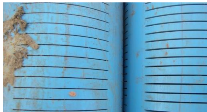
Figure 4: PVC screen (left 0.75mm slot, right 1mm slot)
