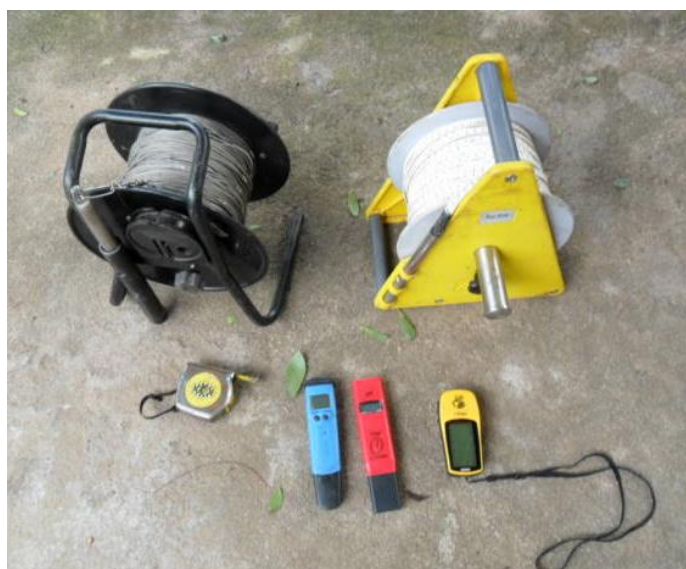
Figure 1: Some kit – depth meter, electronic dipper, tape, EC and PH meters, Global Positioning System (GPS)
