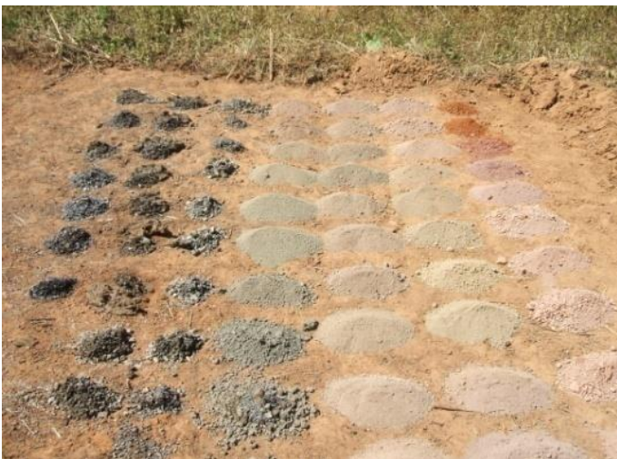
Figure 6: Samples are laid out and logged for 1m depth intervals
