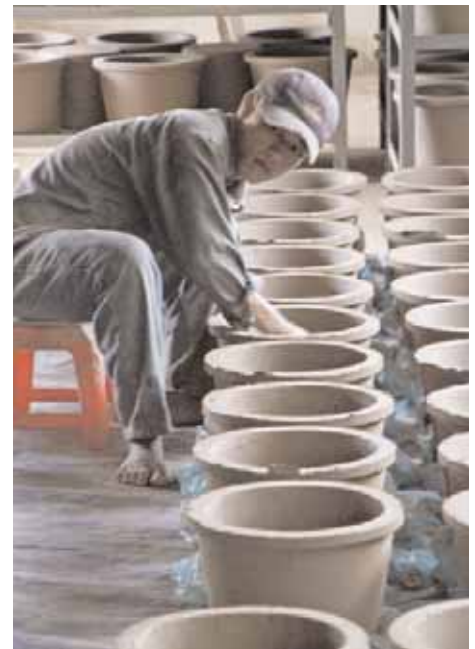
Pots are inspected and smoothed manually after pressing
