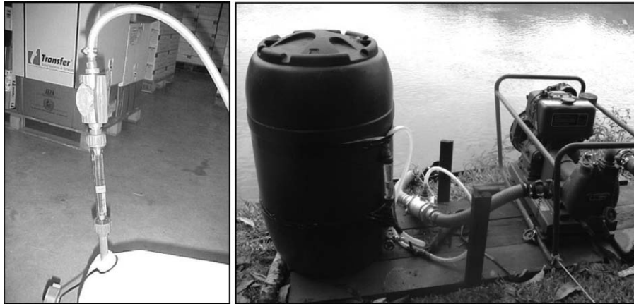
Fig. 4. Different suction side doser configurations as used by MSF (left) [12] and Oxfam (right) [16].
