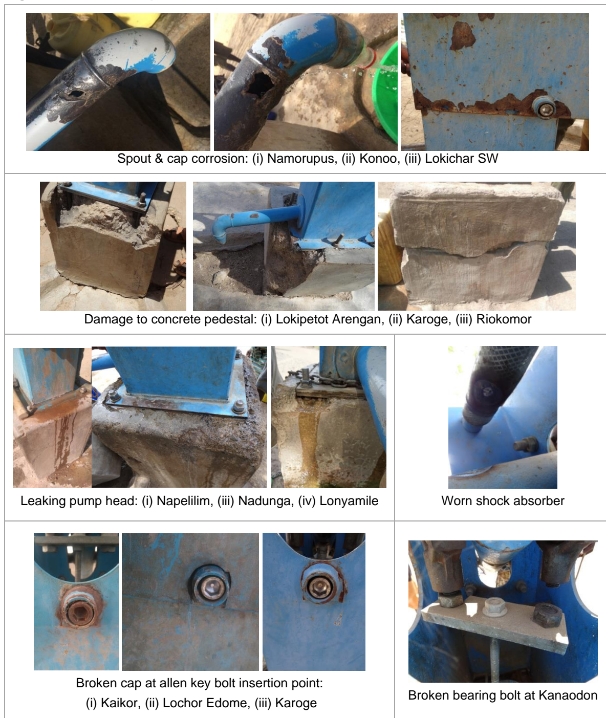
Figure 10 - BluePump wear and tear in Turkana
