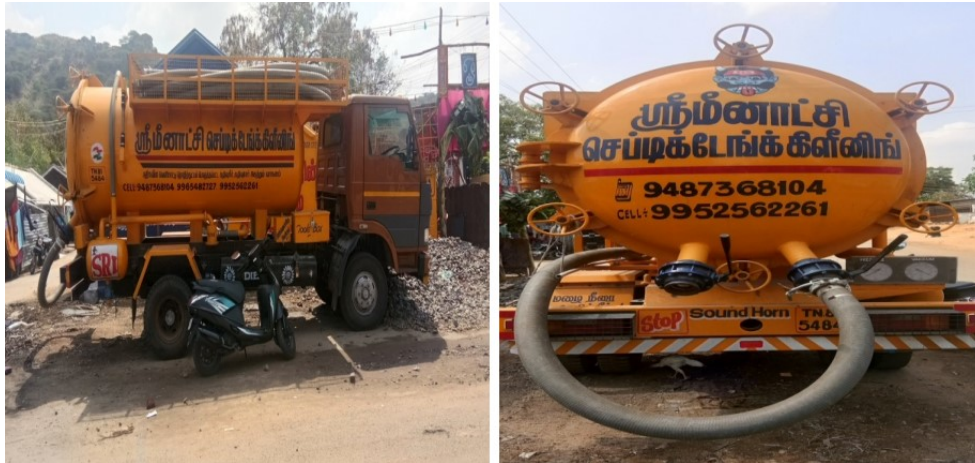
Figure 5: Emptying of a septic tank.
