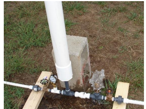
Figure 14. A 3/4-inch hydraulic ram pump (Design 1) in operation. The image was taken just at waste valve closure. The concrete block is in place to support the air chamber. Image credit: W. Bryan Smith, Clemson University.
