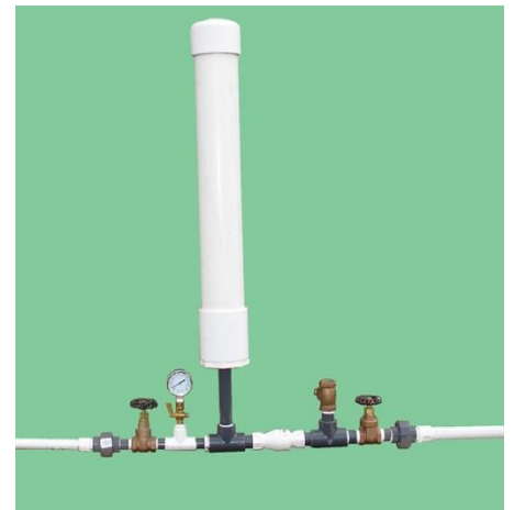
Figure 1. A 3/4-inch homemade hydraulic ram pump made with PVC fittings. Water flows from right to left during operation. Image credit: W. Bryan Smith, Clemson University.
