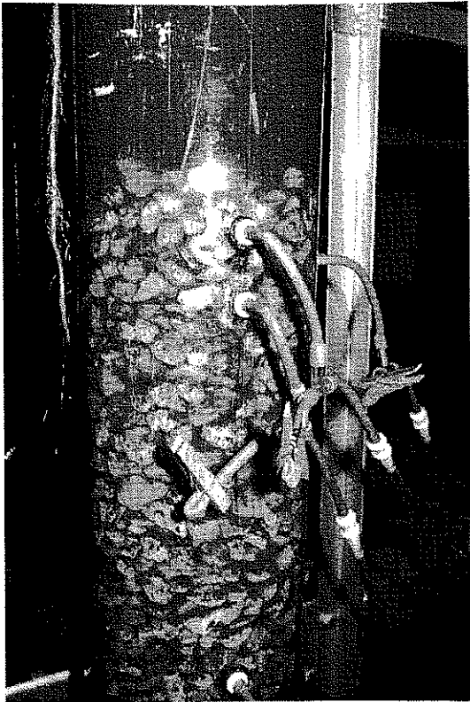
Photo 7 Vertical Roughing Filter Column
