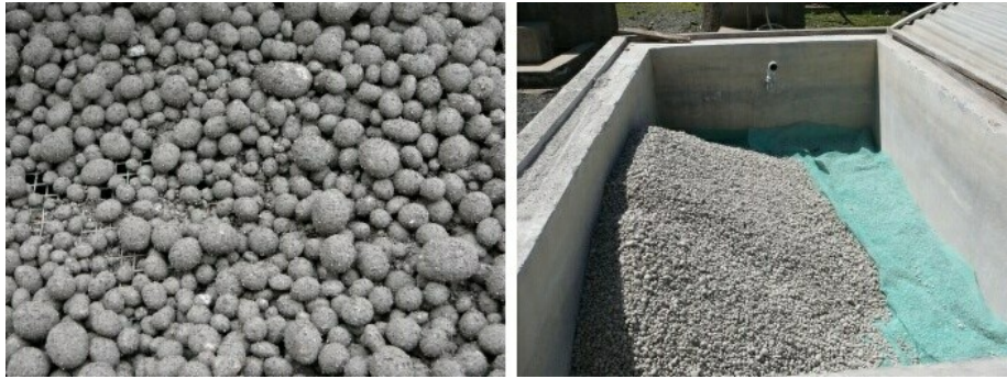
Fig. 7.9 Calcium phosphate pellets that are used in combination with bone char in fluoride removal filters (“Nakuru Technique”)
