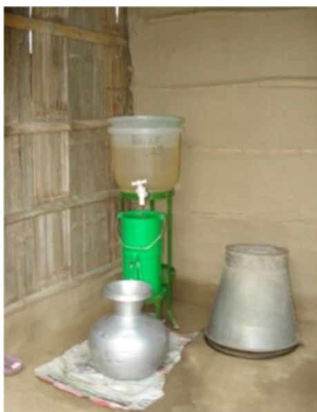
Fig. 7.2 READ-F household ion-exchange filter used in Bangladesh (see also document on “Verified Arsenic Removal Technologies in Bangladesh”)
