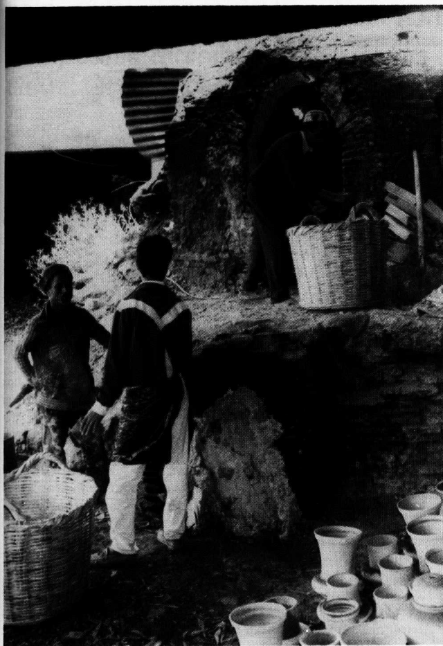
Fig. 4. A Moroccan beehive kiln is unloaded. In the foreground, clay used to cover its fire chamber can still be seen.
