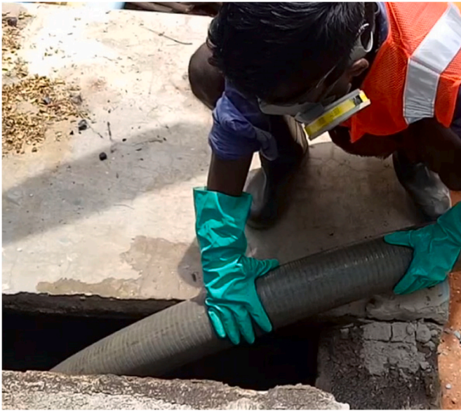
Fig. 5. Images of field testing of the PPE - Inserting a hose pipe.
