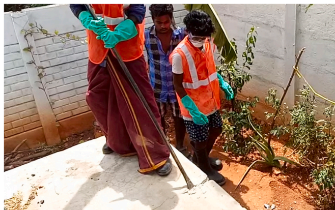
Fig. 4. Images of field testing of the PPE- Opening a septic tank.
