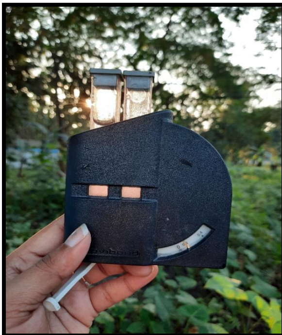
Image 1: Free Residual Chlorine concentration in water sample collected from nearest street standpost (SSP) – Samuktala PWSS, Alipurduar
