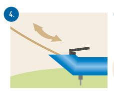
→ Use the rod to control brushing of the interior of the pipe.
