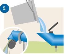
→ After brushing both ends of the WASHaLOT, flush the dirty water and rinse the pipe with clean water until it is clean.
