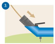
→ Insert the brush through the water inlet of the WASHaLOT.
