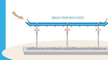
→ Insert the brush through the water inlet of the WASHaLOT.
