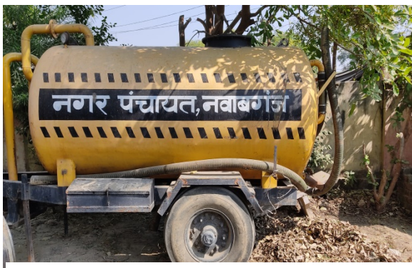
Figure 5: ULB owned vacuum tanker.
