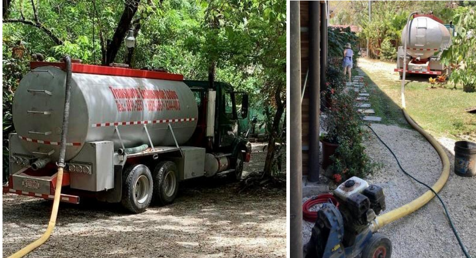
Figure 5: (Left) Vacuum truck equipped with a suction hose from a private company that operates in the area. (Right) Same truck emptying a tank. Source: (Sanitarios La Pampa, 2021).
